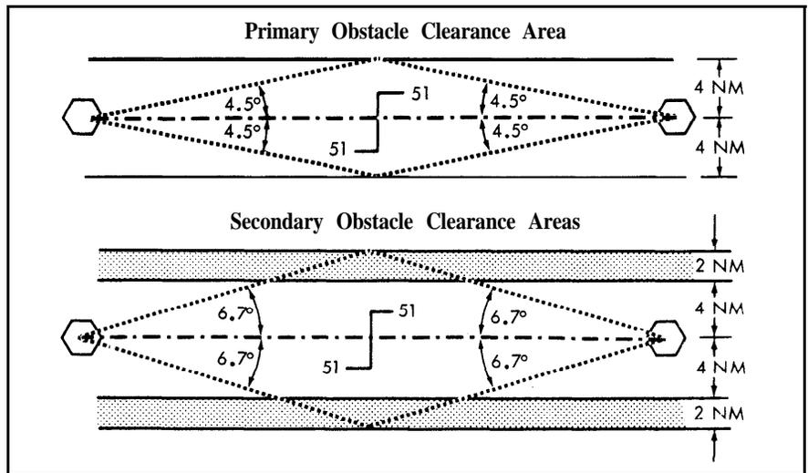
**Figure 2.** At 51 miles from the VOR, the combined six-mile width of the primary and secondary areas represents 6.7 degrees, which is the VOR along-track error limit. Beyond 51 miles, the secondary area expands at 6.7 degrees, as the primary expands at 4.5 degrees.
