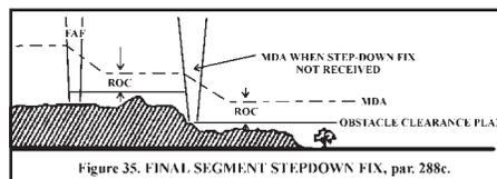
Figure 7. Application of final-segment step-down fix criteria where minimums are to be published both for reception and non-reception of the step-down fix.
