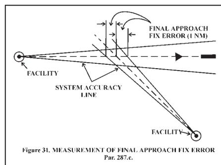
Figure 2. The intersection-fix FAF cannot normally have more than one mile of error on the worst side of the fix.
