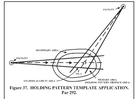
Figure 10. TERPs holding pattern criteria at an intersection fix. At least three of the four corners of the fix displacement area must be contained within the primary area of the holding pattern template. Holding at a "fuzzy" intersection is betting that navigation system errors are both random and correctly quantified.
