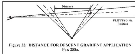
Figure 3. Application of intersection-fix error assumptions for descent gradient application.
