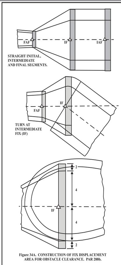
Figure 34A. CONSTRUCTION OF FIX DISPLACEMENT AREA FOR OBSTACLE CLEARANCE. PAR 288b.
