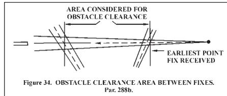
Figure 4. Application of intersection-fix error assumptions for obstacle clearance area.
