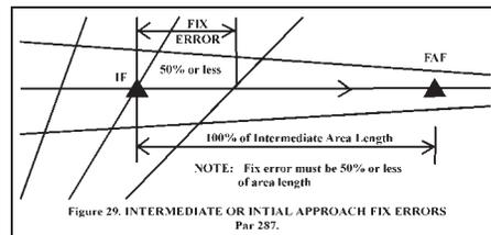
Figure 1. The intersection-fix IAF or intermediate fix can be so sloppy as to consume up to 50 percent of the length of the succeeding intermediate segment.
