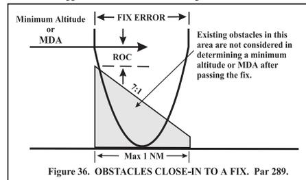
Figure 6. Obstacles located in the final approach area within 1 mile past the point where a fix can first be received may be eliminated from consideration by application of a descent gradient of 1 foot vertically for every 7 feet horizontally.
